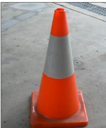
Orange: Works limit marker cone
